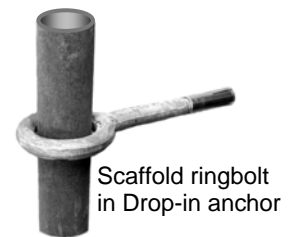
"Drop-in" internally threaded, hammer set expansion socket anchor - for concrete
